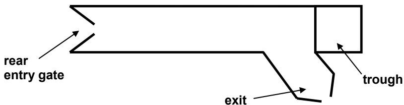
Figure 1. Mechanics of an electronic sow feeder (ESF).
